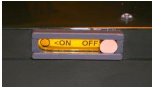
3. Switch the magnet slowly back and forth between **OFF** and **ON** a few times; continue until the lamp flashes blue once. Now leave the magnet switched to **ON**.
